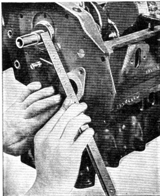
Fig. 25—Checking Alignment of Timing Gears
