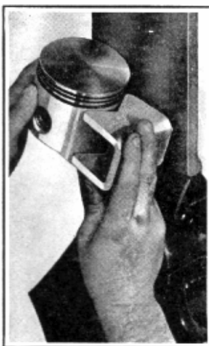
Fig. 40—Checking Piston and Connecting Rod Assembly for Twisted Connecting Rod
