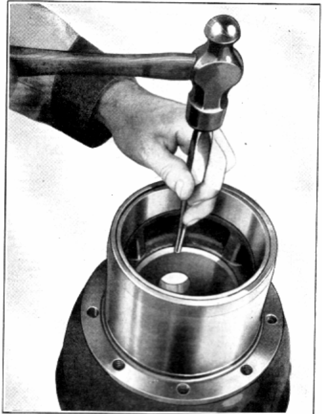
Fig. 15—Removing Inner Bearing Outer Race
