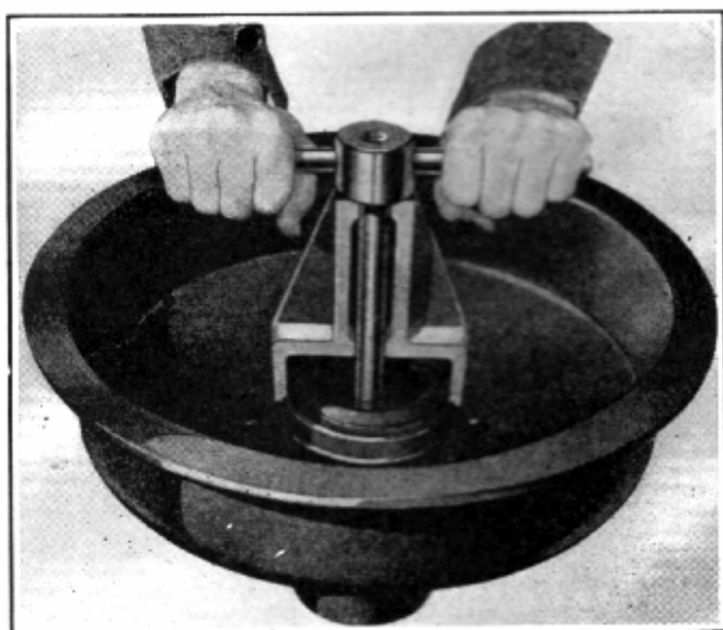
Fig. 3—Removing Inner Bearing and Oil Seal
