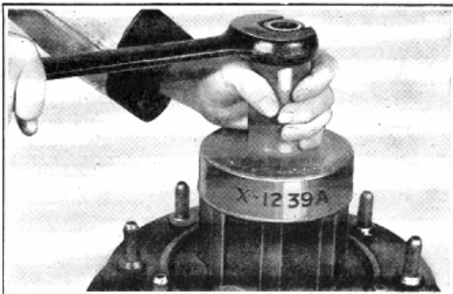
Fig. 27—Removing Outer Bearing Race Using Tool No. X-1239-A
