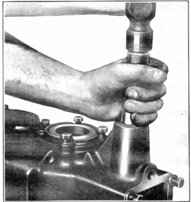
Fig. 37—Installing Shift Shaft Oil Seal, Tool No. J-1723
