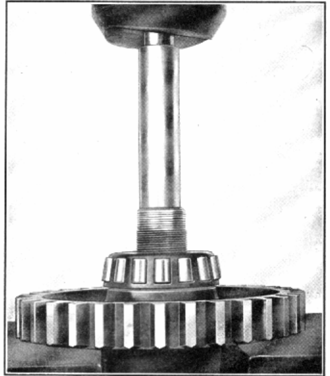
Fig. 21—Pressing off Idler Shaft Gears and Bearings
